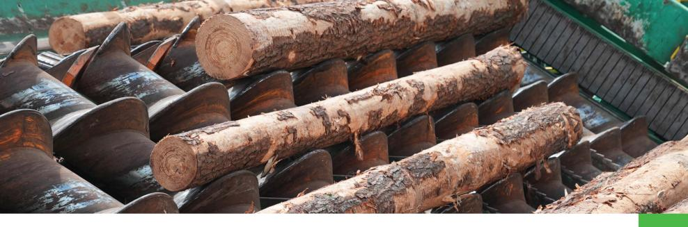
SPRINGER's innovative screw technology transports the logs onward in the screw system without chains. It stands out for its low noise, optimum efficiency, and high speeds when feeding log sorting systems and saw lines.
