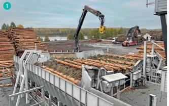
ufacturer installed cameras instead of sensors in the entire infeed area. The cameras detect the logs from above and pass the information on to the system control, which guarantees an optimal material flow. Seven robustly designed screw feeders, which enable small gaps between logs in
