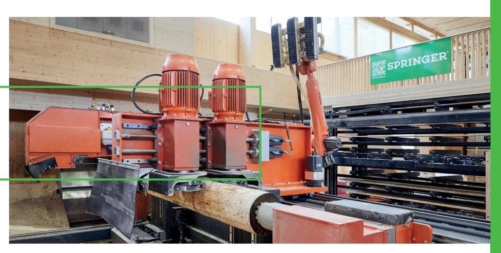
The SAWBOX redefines standards for log production. Its compact design centralizes all processing steps in one center, ensuring efficient production with minimal space needs. Unlike traditional sawmills, it streamlines processing into a single step, allowing for efficient production with only one operator.
