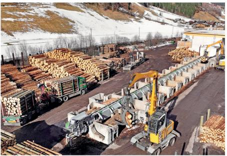
port and sort logs with a diameter of 100 mm to 800 mm and a length of 3.1 m to 5.3 m.
